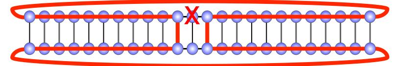
When node down occurs, torus connection can be kept by the redundant links.
