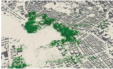
Figure 12.7: Q-criterion ( $Q=0.0015$ ) in Shiodome area
