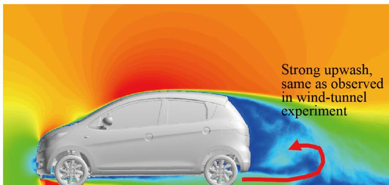
Figure 12.4: Overview of characteristic flow field (SUZUKI MOTOR CORPORATION).
