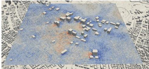
Figure 12.6: Pressure field in Marunouchi area(50m Height)
