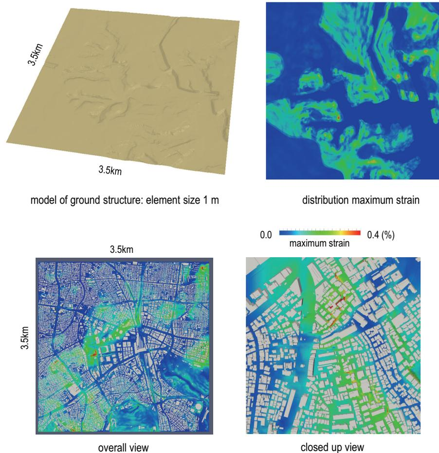
Figure 17.4: Example of ground deformation distribution and induced lifeline damage
