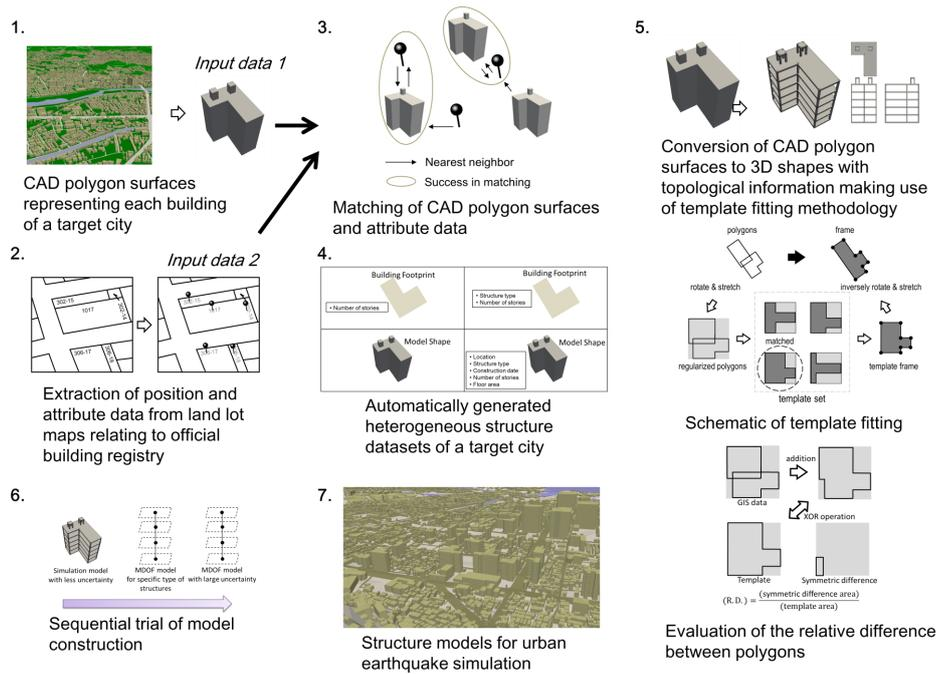
Figure 17.2: Platform of processing data resources to generate urban area model
