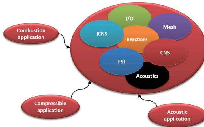
**Figure 1. Framework of the unified solver CUBE.**
