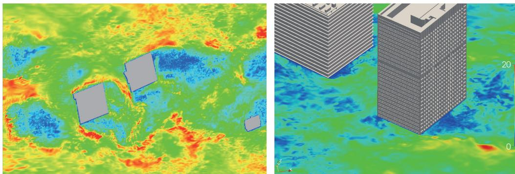
**Figure 8. Detailed flow result showing specific building, showing the interaction of vortex and structure.**
