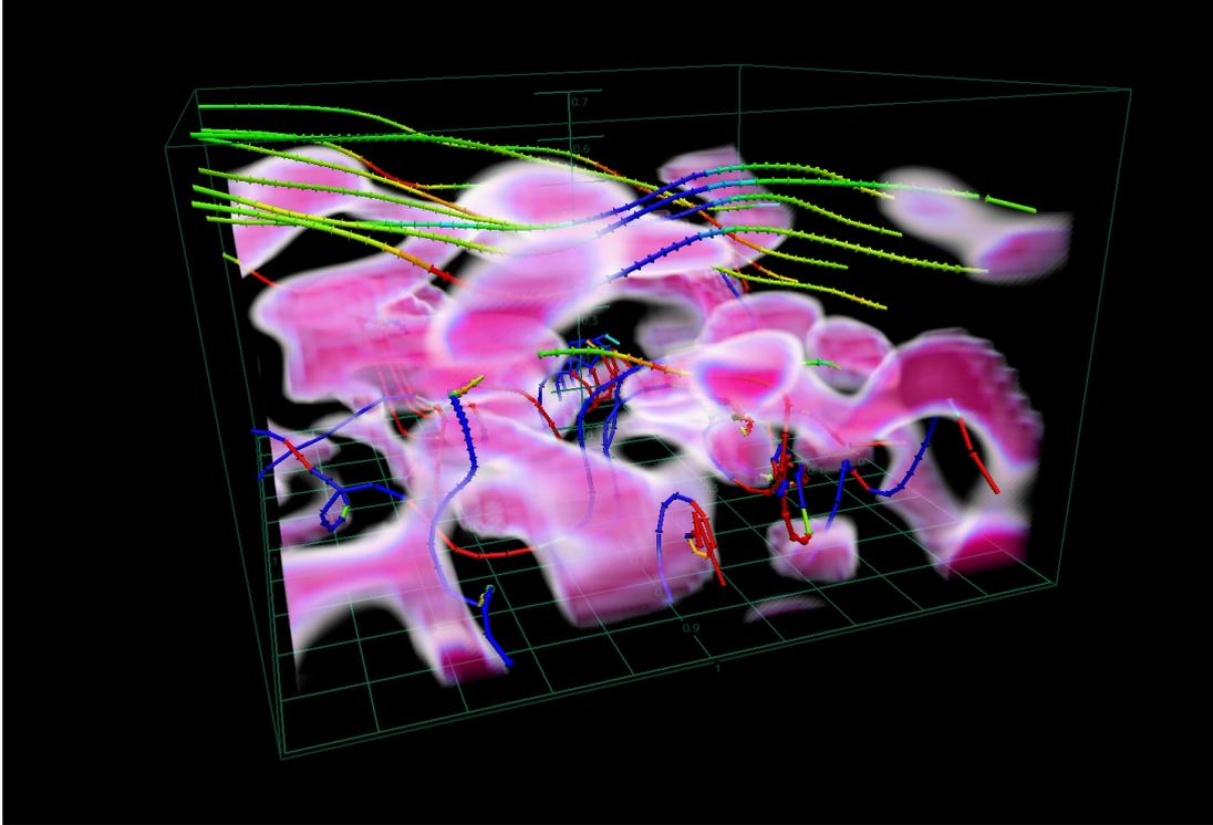
Figure 1. A snapshot of planetary boundary layer simulation with the 25m isotropic resolution. The isosurface and vector indicates the anomaly of potential temperature form the environment and velocity vector, respectively.
