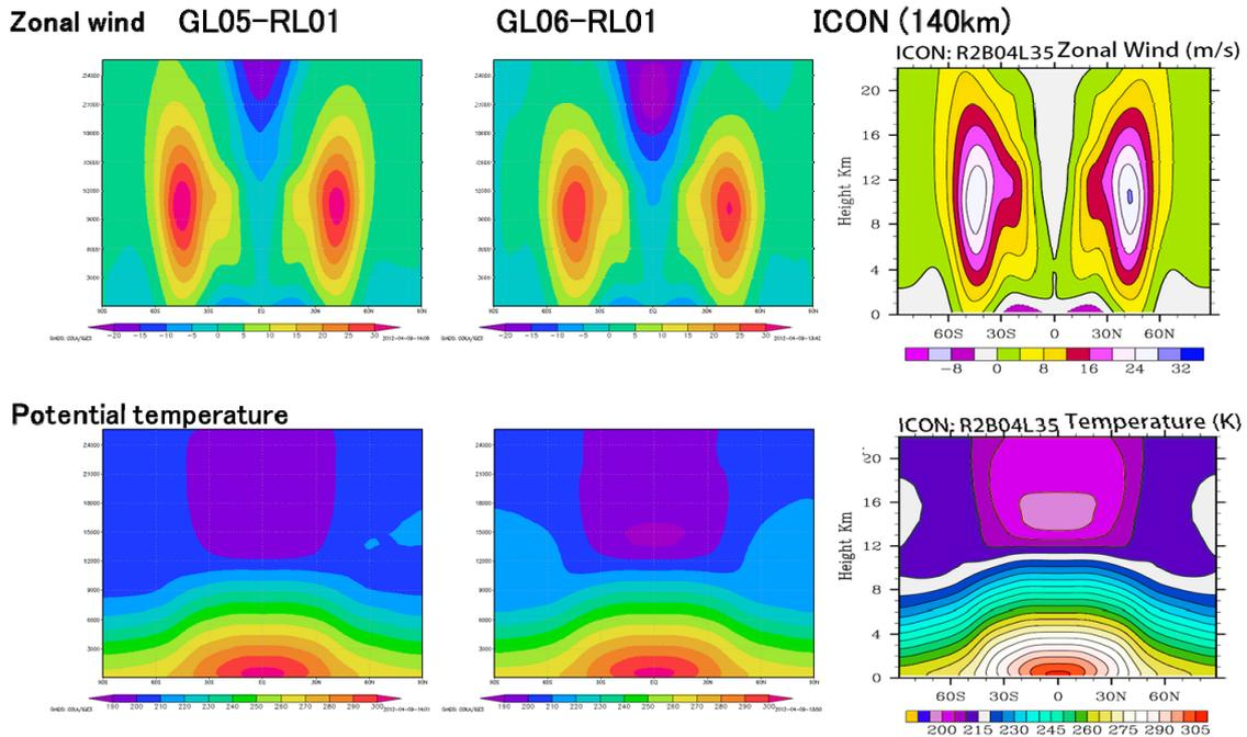
Figure 3. The inter-comparison for Held & Suarez Test Case. Climatology of zonal wind and temperature.
