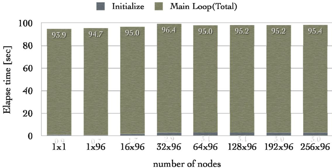
Figure 2. The scalability (weak-scaling) of SCALE-LES on K Computer.
