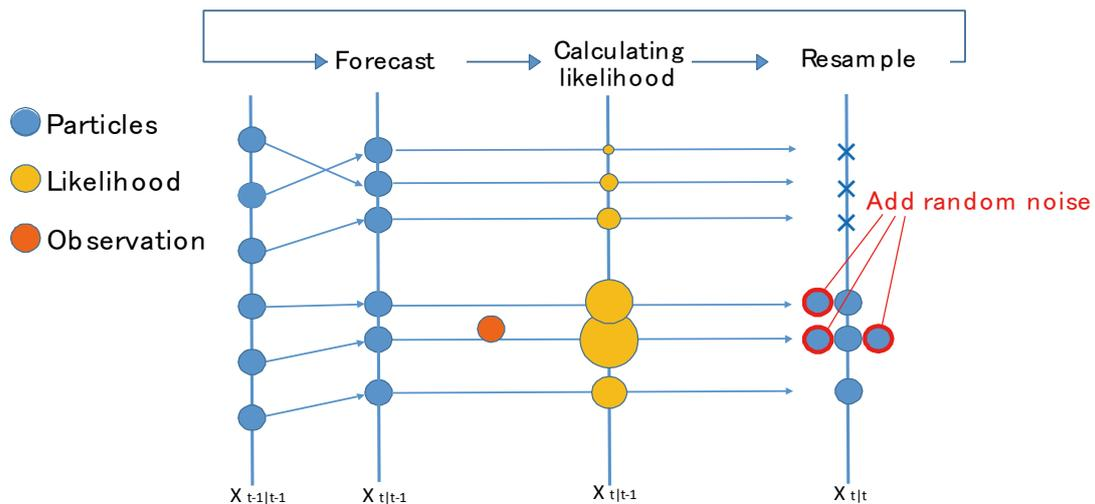
**Figure 7. Schematic showing a sequential importance sampling (SIR) particle filter.**
