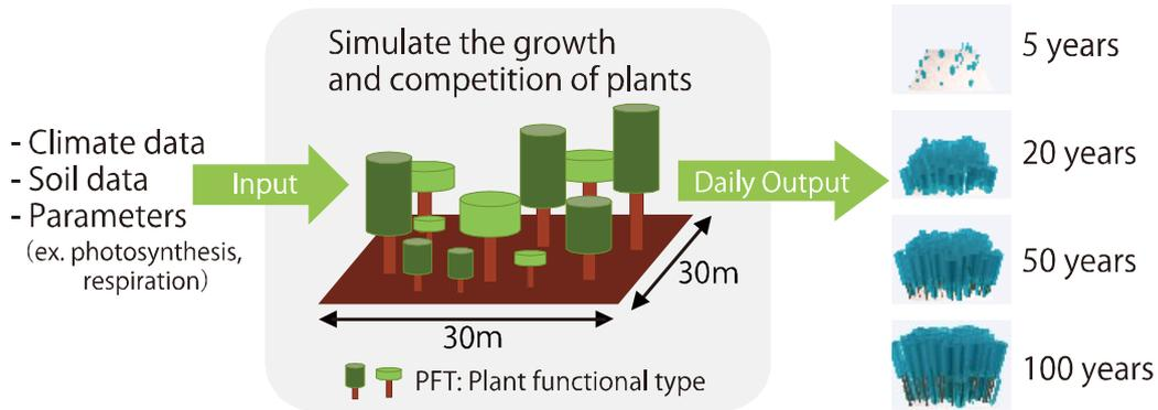
**Figure 6. Schematic of vegetation simulation with SEIB-DGVM.**
