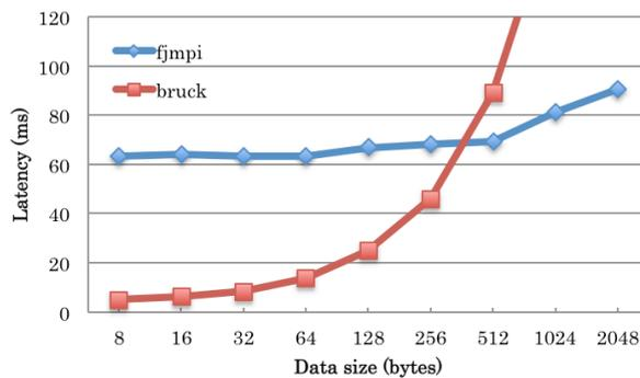
Fig. 2 Comparison of data shuffling time on 16384 nodes. The blue line shows the performance when using an all-to-all API of the Fujitsu MPI, while the red line shows the performance using the custom collective communication.
