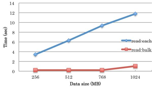
Fig. 1 Read latency comparison on 192 nodes. The blue line shows the read time when all nodes simultaneously read the data, while the red line shows the performance when only a part of the nodes load the data from the local storage, which are then transferred to the rest of the nodes by using MPI over the Tofu network.
