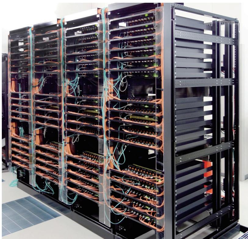
**Fig. 3. MDGRAPE-4 system with 512 chips in 64 subracks.**
