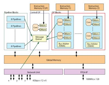
Figure 2. Block diagram of MDGRAPE-4 SoC.
