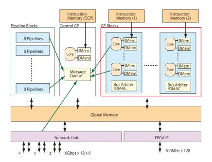
Fig. 2. Block diagram of MDGRAPE-4 SoC.
