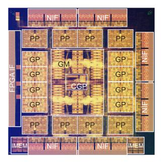
Fig. 3. Layout image of MDGRAPE-4 SoC.
