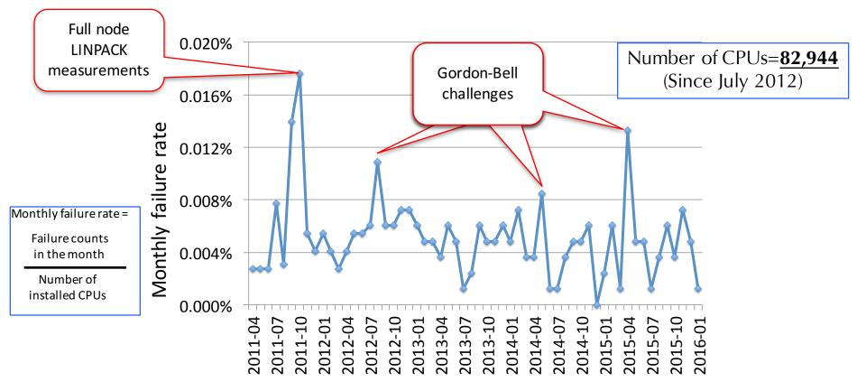
Failure trend of CPUs is almost stable except after high load events
