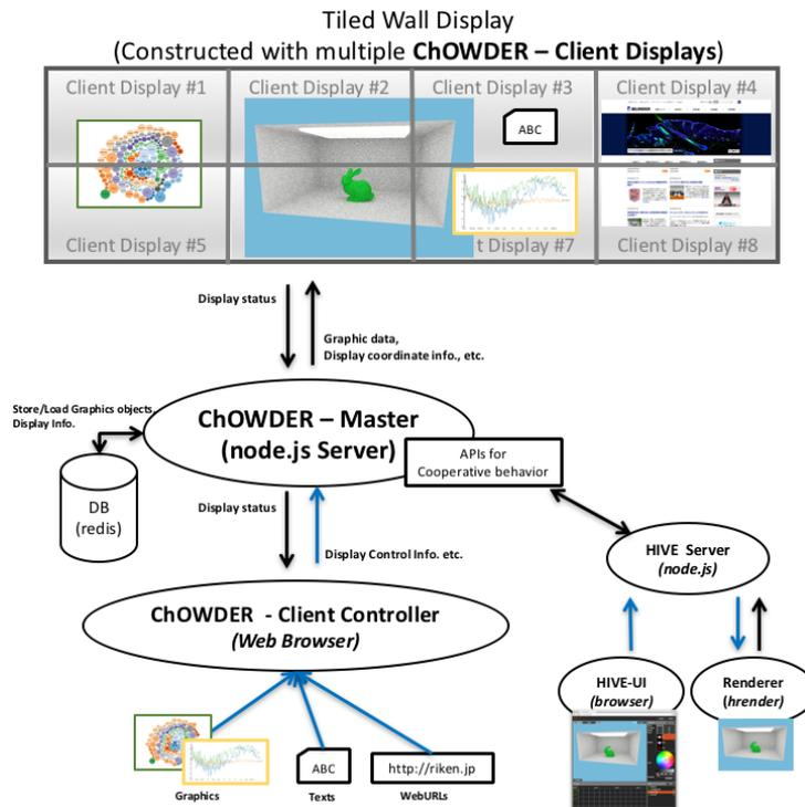
Figure 14.7: System diagram of ChOWDER.
