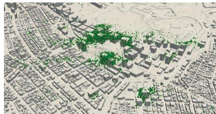
Figure 12.8: Q-criterion ( $Q=0.0015$ ) in Marunouchi
