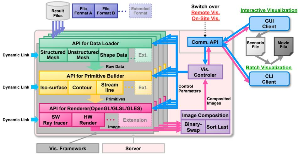
Figure 2: Logical design of a LSV system. Switching over the connection of modules, the LSV provides various operating scenarios for users.
