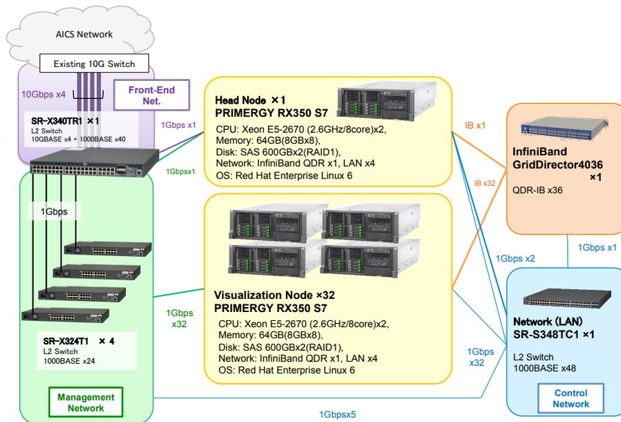
Figure 1: Configuration of an installed visualization cluster system.
