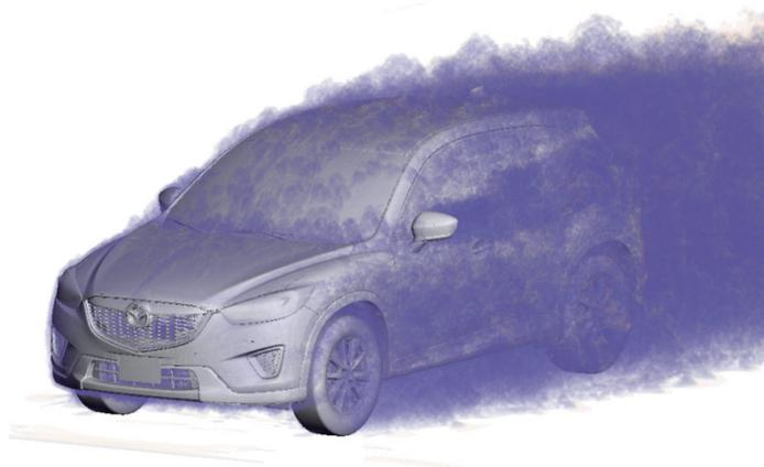
**Figure 5. Flow visualization results of vortex structure**
