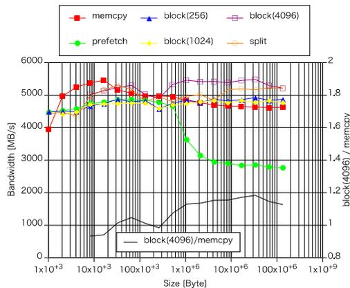
Figure 8. Multi-threaded memcpy bandwidth over region size
