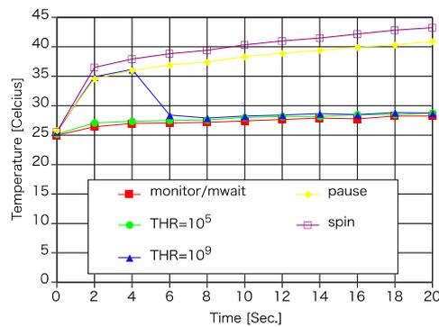
Figure 7. CPU temperature over time while synchronization
