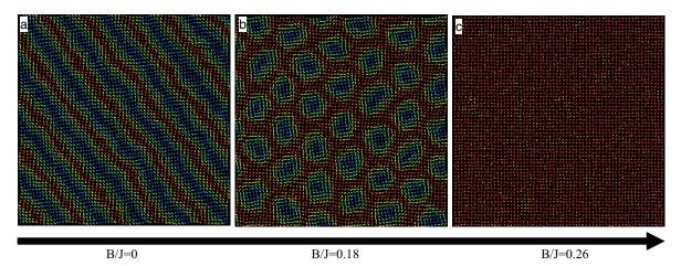
Fig. 6: Phase transition from (a) helical order to (b) Skyrmion crystal and to (c) ferromagnetic order with increasing external magnetic field B/J in 2D squared lattice with 128×128 spins.
