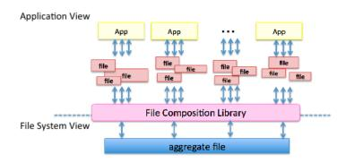
Figure 1. Concept of the file composition technique
