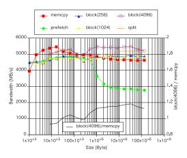
Figure 8. Multi-threaded memcpy bandwidth over region size
