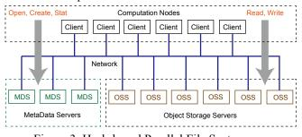
Figure 3. Hash-based Parallel File System
