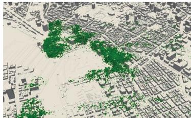
Figure 12.7: Q-criterion ( $Q=0.0015$ ) in Shiodome area
