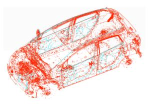
Fig. 2 Data defecting points in a CAD (red: gap, and cyan: overlap of two parts).
