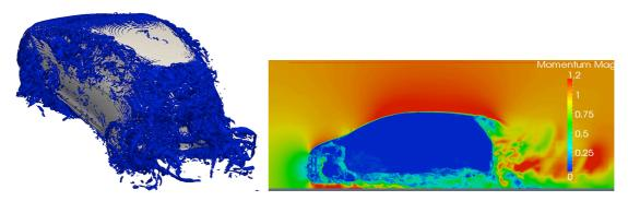
Fig. 4 Flow structures (left) and the magnitude of flow-velocity around the vehicle.
