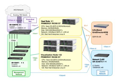
Figure 1: Configuration of an installed visualization cluster system.
