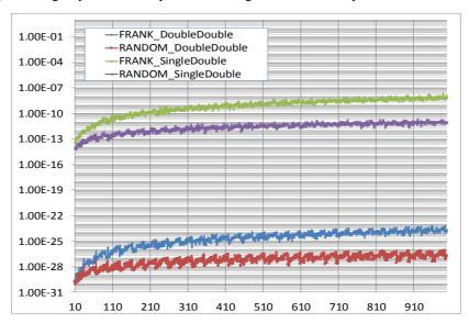
Figure 4: Accuracy test of QPEigenK on a Fujitsu FX10 (Absolute Residual Error max|Ax-wx|\_oo)
