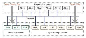
Figure 6 Hash-based Parallel File System
