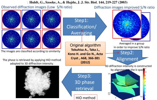
Figure 2 Obtaining electron density map from XFEL snapshots
