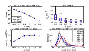
dependences Figure Resolution convection characteristics: (a) the number of convection, (b) the maximum vertical velocity, (c) the ratio of the area of convection core to that of convective grids, and (d) the grid distance to the nearest convection. The thin—dashed line in (a) indicates log x4 as a reference. GL08 denotes 30 km horizontal resolution, while GL13 indicates 0.8 km resolution.
