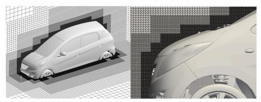
Fig. 3 BCM mesh generated around a full-scale vehicle using about 150 million cells.
