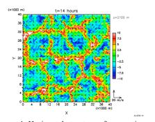
Figure. 4, Horizontal structure of convective cell at height of 2.1km in a Marian planetary boundary layer experiment. Color tone and vector show vertical velocity and horizontal velocity,
