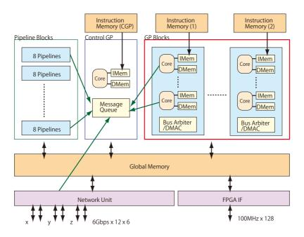
Fig. 2. Block diagram of MDGRAPE-4 SoC.
