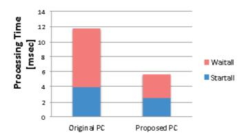
Figure 8 Comparison of original persistent communication and proposed one.
