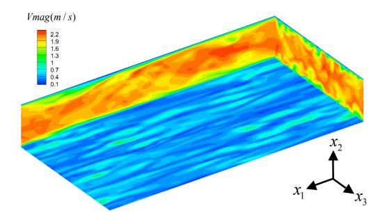
Figures 8. The instant contour of the velocity magnitude
