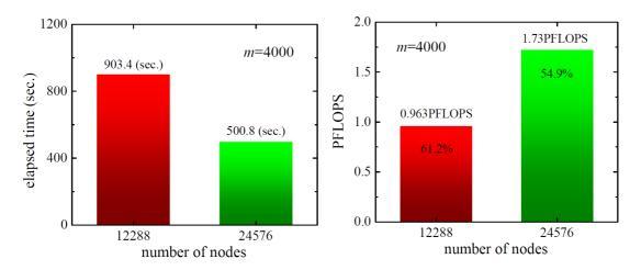
Fig. 3: The elapsed time (left) and the computational effeciency (right) using 12288 nodes and 24576 nodes on the K-computer. This benchmark is performed by the dynamical DMRG calculations on the one-dimensional extended Hubbard model using m=4000.
