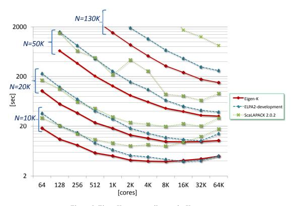
Figure 5: Eigen-K, strong scaling on the K computer
