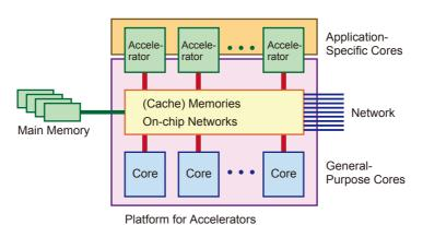
Fig. 1. Diagram of platform for accelerators.
