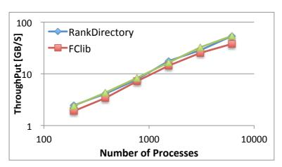
Figure 5 Write throughput of FClib
