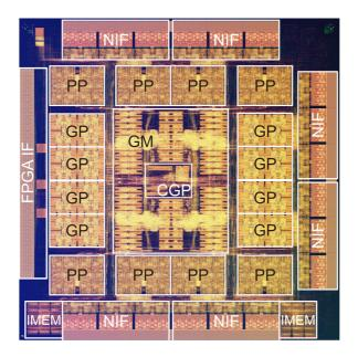
Fig. 3. Layout image of MDGRAPE-4 SoC.
