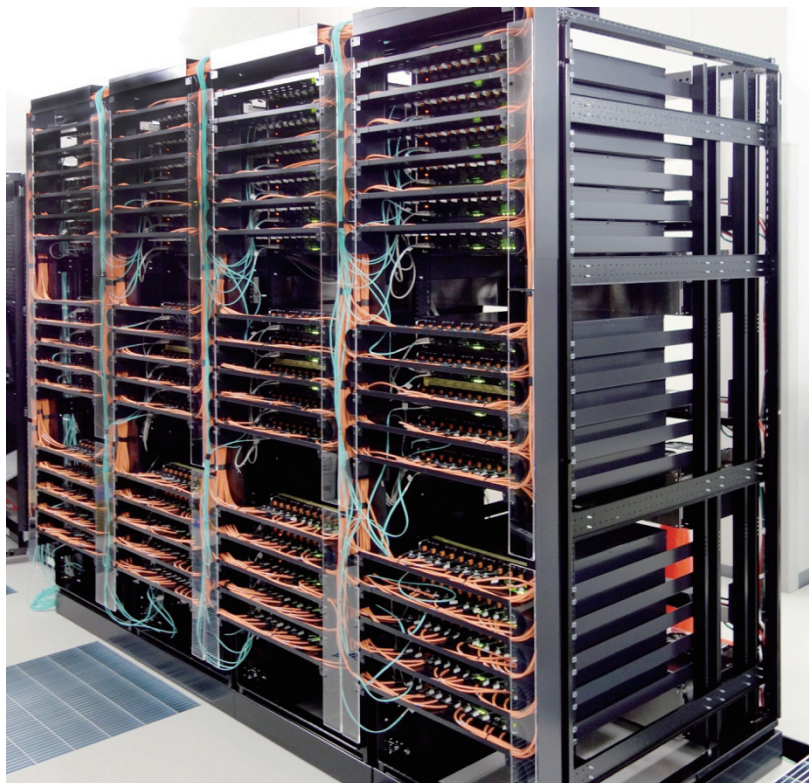
Fig. 3. MDGRAPE-4 system with 512 chips in 64 subracks.
