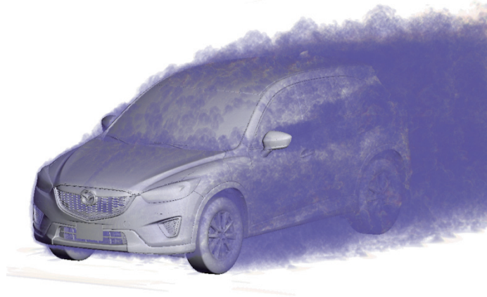
Figure 5. Flow visualization results of vortex structure
